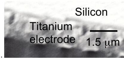
Fig. 4: SEM photo of silicon deposited on the pixel shown in Fig. 3a.
