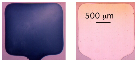
Fig. 3: (a-left) Powered cathode pixel in an array, after 5 min. of deposition at 1.2 Torr, and 300 °C; (b-right) un-powered cathode pixel from the same array
